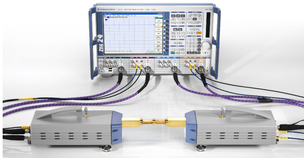
Test setup for 2-port transmission measurement with R&S ZVA-Z110 (similar for the other models)
